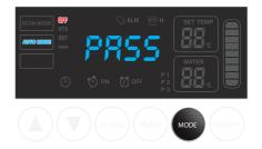
2. Press 'UP ARROW' to change 'PASS' to '0000'. To enter the password, adjust each number using the 'ARROW' buttons and select 'TIMER' to confirm. When the password has been correctly entered, press 'TIMER'. 'F11' will appear on the display.
